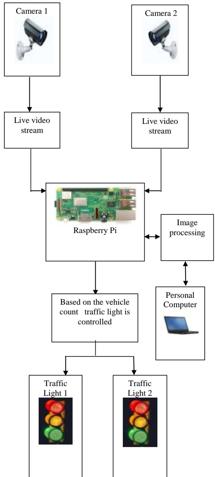
Figure.1 Block diagram of Smart Traffic Light Control System
