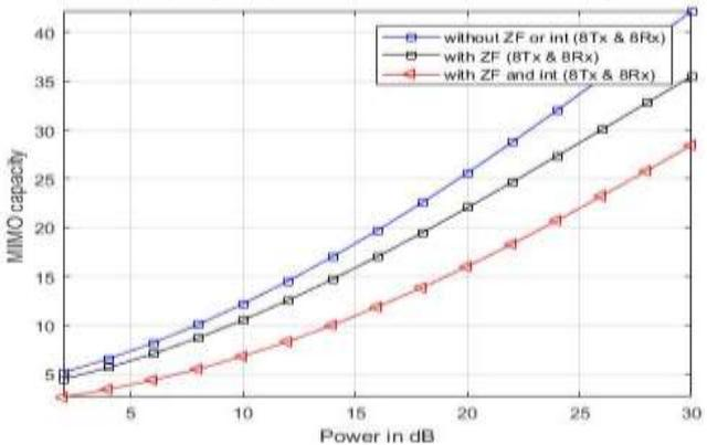
Figure 3: Capacity (Mbps) vs. Power (dB) for 8x8 MIMO systems
