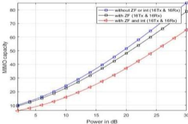
Figure 4: Capacity (Mbps) vs. Power (dB) for 16x16 MIMO systems
