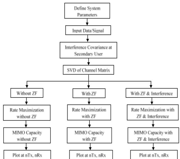
**Figure1.** Block Diagram of the Proposed Technique
