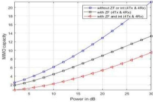
Figure 2: Capacity (Mbps) vs. Power (dB) for 4x4 MIMO systems
