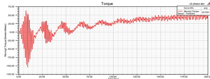
Fig. 18 Torque response of Induction Motor over period of Time during fault condition with three coils open of stator winding
