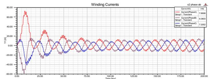
Fig. 14 Current response of Induction Motor during fault condition with two coils open of stator winding
