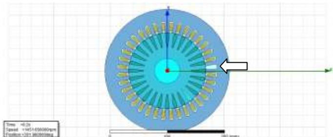
Fig. 6 Model of Induction Motor with one coil of phase A open of stator winding
