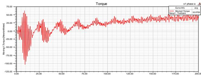
Fig. 8 Torque response of Induction Motor over period of Time during fault condition with one coil open of stator winding
