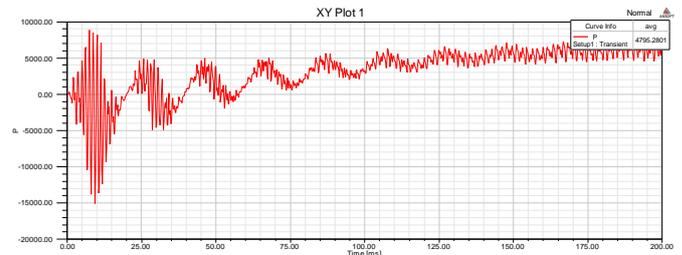
Fig. 5 Output Power response of Induction Motor during normal condition
