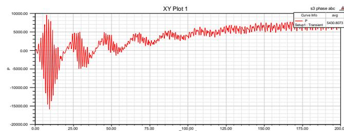
Fig. 20 Output Power response of Induction Motor during fault condition with three coils open of stator winding
