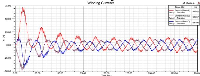
Fig. 9 Current response of Induction Motor during fault condition with one coil open of stator winding
