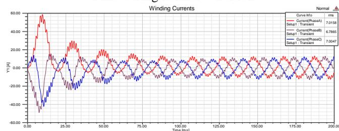
Fig. 4 Current response of Induction Motor during normal condition
