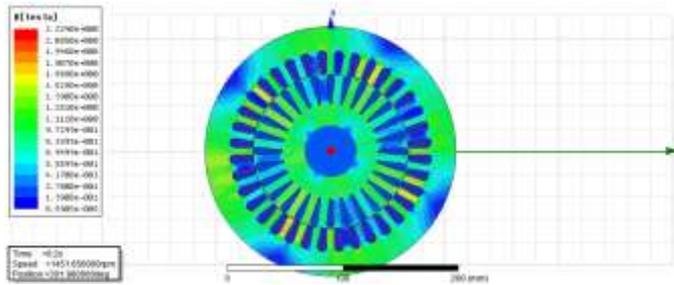
Fig. 17 Flux density distribution of Induction Motor during fault condition with three coils open of stator winding
