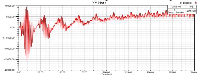
Fig. 10 Output Power response of Induction Motor during fault condition with one coil open of stator winding
