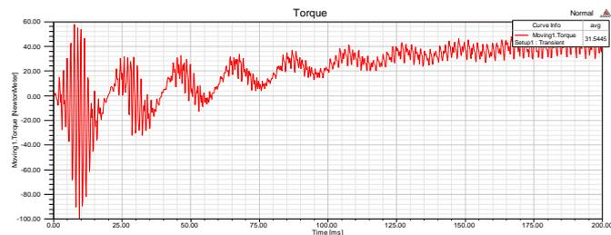
Fig. 3 Torque response of Induction Motor over period of Time during normal condition
