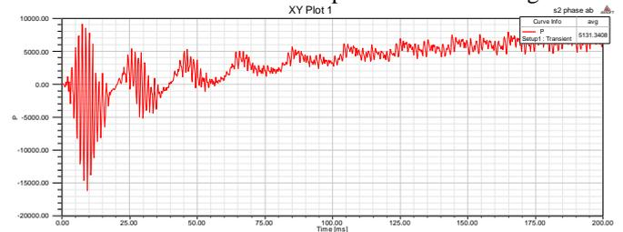
Fig. 15 Output Power response of Induction Motor during fault condition with two coils open of stator winding
