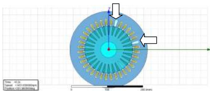
Fig. 11 Model of Induction Motor with two coils open of stator winding
