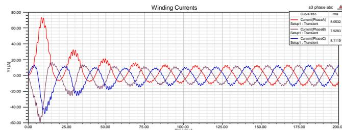
Fig. 19 Current response of Induction Motor during fault condition with three coils open of stator winding
