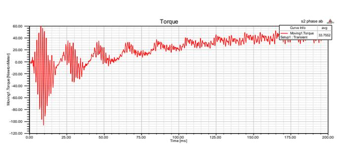
Fig. 13 Torque response of Induction Motor over period of Time during fault condition with two coils open of stator winding
