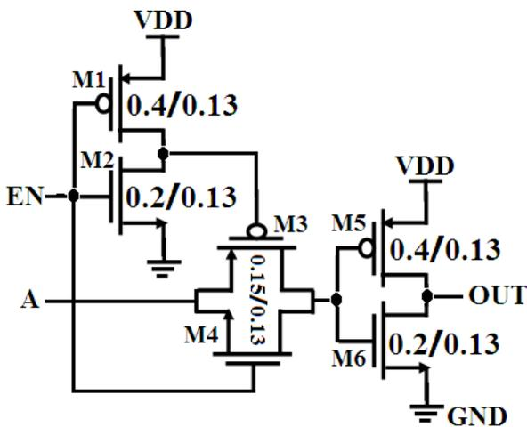
Figure1. Proposed tri-state inverter circuit using TG logic.
