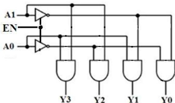
**Figure8.** Schematic diagram of a 2-to-4 static decoder.
