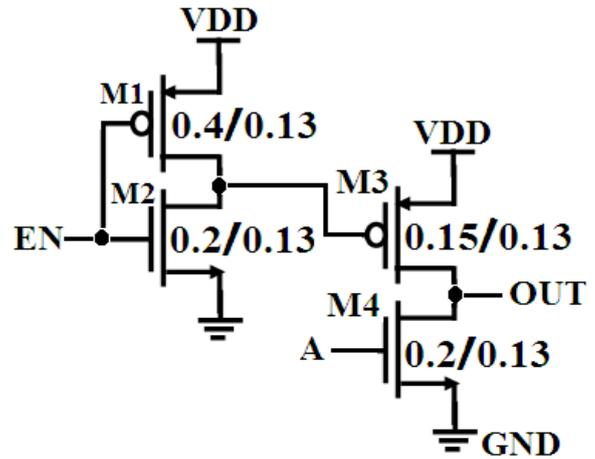
Figure2. Proposed tri-state inverter circuit using pseudo-nMOS logic.
