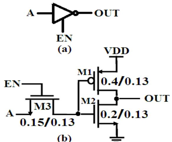
Figure3. (a) tri-state inverter logic symbol (b) Proposed tri-state inverter circuit using PT logic.
