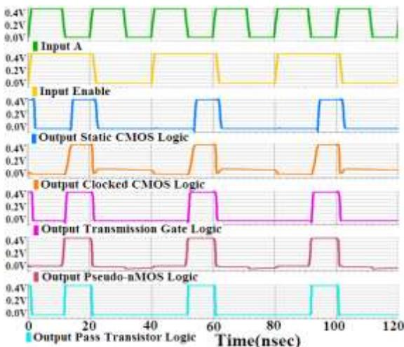
Figure4. Simulated waveform of the available and proposed tri-state inverters.
