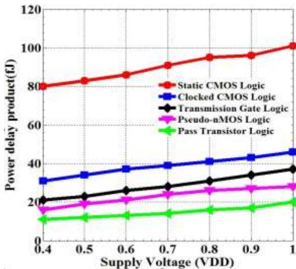
Figure6. Power delay product vs. supply voltage of different tri-state inverters.
