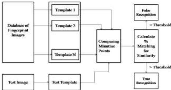
Figure3. Block diagram of Fingerprint Matching
