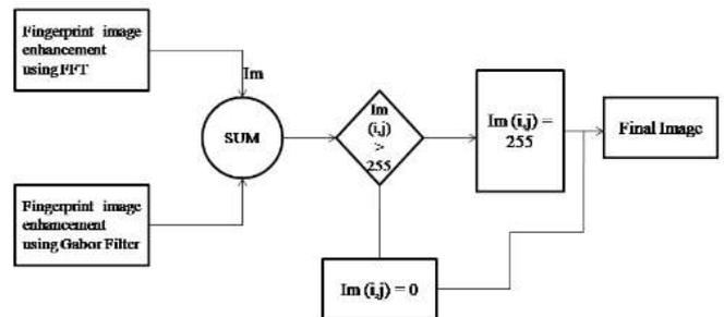
Figure2. Block Diagram of Enhancement Technique
