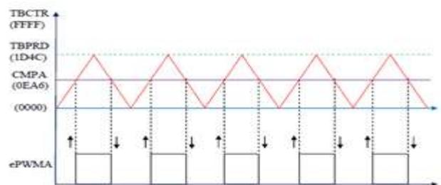
Fig.5 PWM Wave generation by ePWM module
