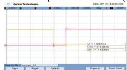
Figure11.Dead Band between normal & inverted drive signal
