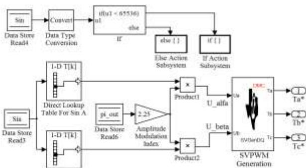
Figure3. MATLAB/SIMULINK Model for Space Vector Sinusoidal Signal Generation
