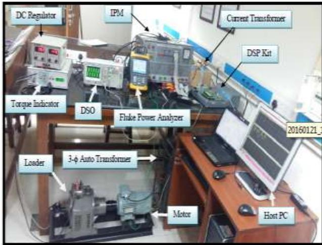
Figure.6 Real Image of Experiment Hardware Setup
