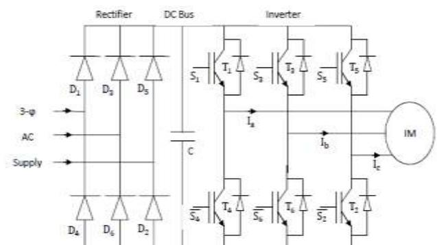
Figure1. IGBT Based Three Phase Inverter Controlled by Six PWM Signals.
