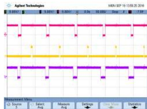
Figure9. SVPWM Output of Three Phases in Small Time-Scale
