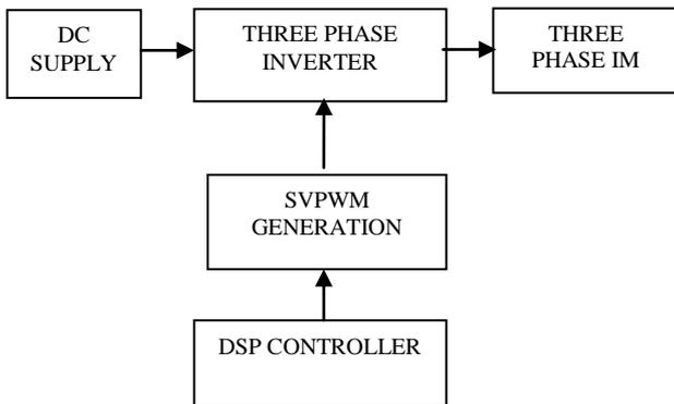
Figure2. Block diagram of PWM switching pulse generation using DSP
