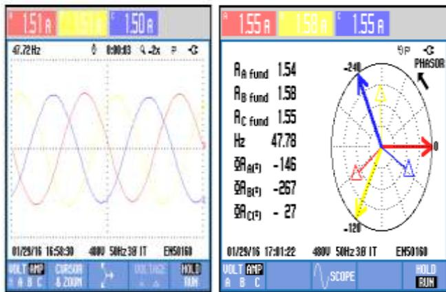
Figure13. Output Phase Current Waveform of IPM using SVPWM Technique
