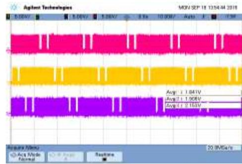
Figure8.SVPWM Output of Three Phases
