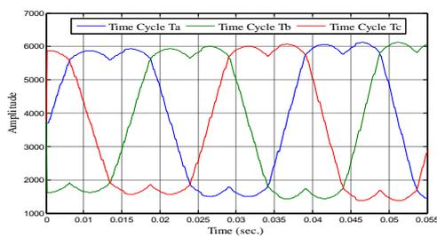
Figure7. Simulated Waveforms of Duty Cycle Ta, Tb, Tc
