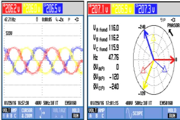
Figure12. Output Phase Voltage Waveform of IPM using SVPWM Technique
