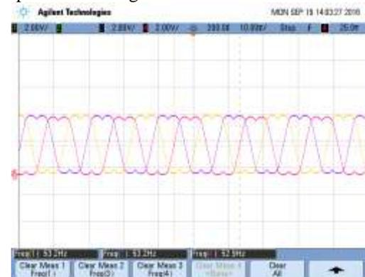
Figure10. Low-Pass Filtered Form of PWM1 PWM2 and PWM5 Pulses
