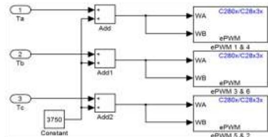
Figure4. SIMULINK Model of ePWM Module for PWM Generation
