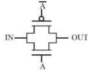
Figure .3. Transmission gate
