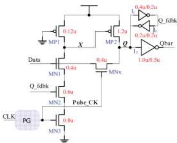
Figure .4. Schematic of the existing P-FF design.
