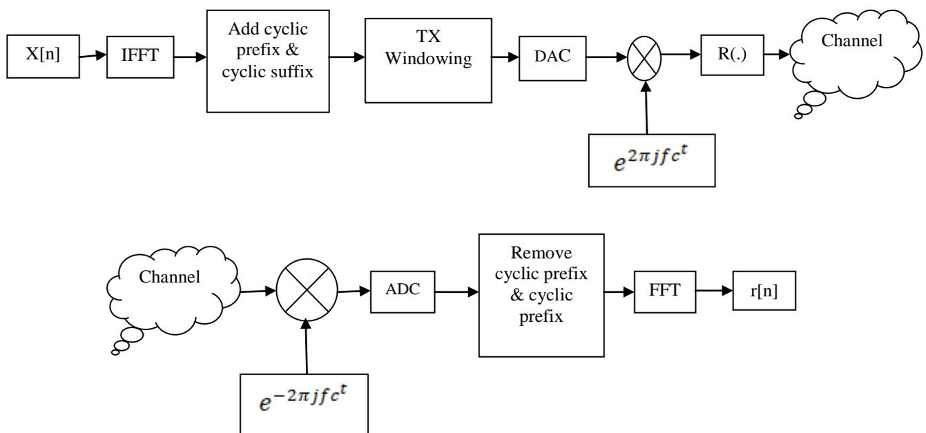
Fig. 1. L-DACS1 core transmission system
