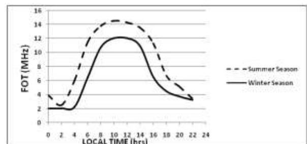
**Figure 1.** The predicted optimum working frequencies (FOTs) chart of the winter and the summer seasons for Tripoli-Benghazi HF radio communications Link, (hrs = hours, MHz = megahertz).
