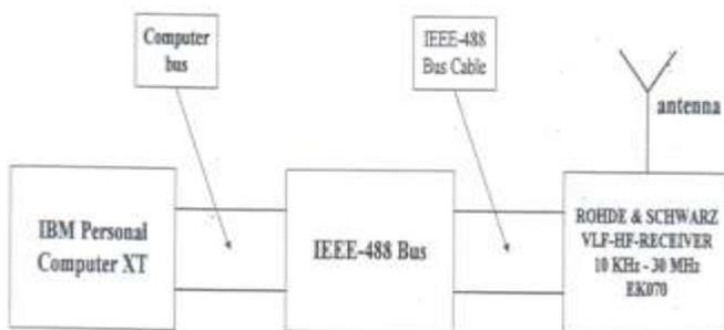
**Figure 2.** A block diagram of the experimental set-up.
