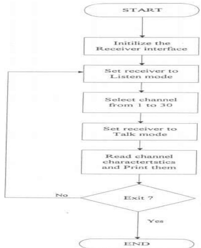
**Figure 3.** The measurements' flow chart of the received short (HF) signal level with its operating frequency of 7.245 MHz.
