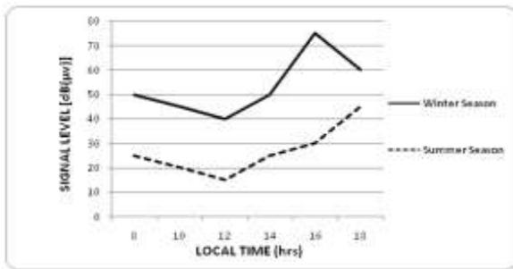
**Figure 4.** The median values of the received short (HF) signal level variations' measurements with an operating frequency 7.245 MHz at Benghazi City - Libya.
