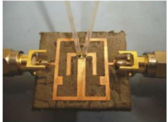
Fig.10. Fabricated prototype of optically reconfigurable Microstrip UWB Bandpass Filter [25]
