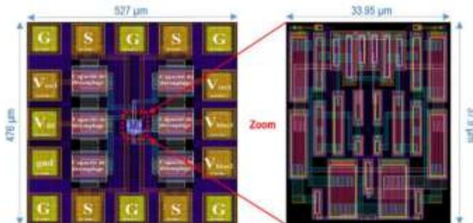
Fig.6. Layout of band-pass filter using tuneable active inductor (TAI) simulated using a 0.13 $\mu$ m CMOS technology [21]
