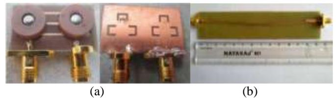
Fig. 2. a) Two pole dielectric resonator band-pass filter [11], b) Micro-strip line based band-pass filter [14].
