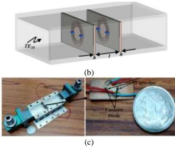
Fig. 8. Dual mode dual band waveguide band-pass filter [23] a) Proposed Varactor diode and chip capacitor loaded planar split ring resonators b) Placement of proposed ring resonator in waveguide c) Fabricated prototype with placement of ring resonator inside WR-90 waveguide.
