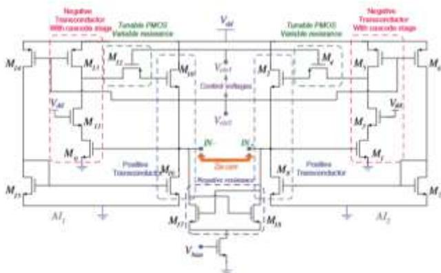
Fig. 5. Schematics of proposed differential TAI [21]
