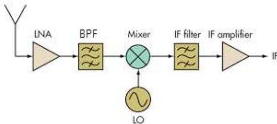
Fig.1. Typical block diagram of wireless receiver system
