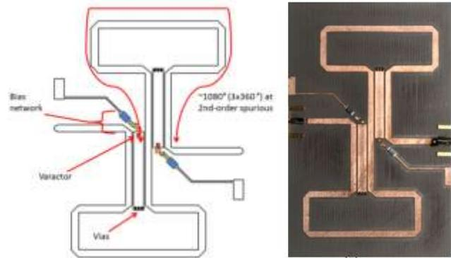
Fig. 3. Tunable band-pass filter using varactor diode [18]
