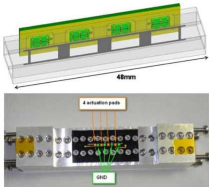
Fig. 9. HFSS simulation model and fabricated prototype of RF MEMS based electrically tunable waveguide filter [24]
