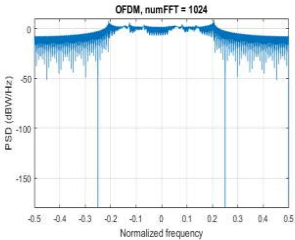
Figure 4: PDS of Typical OFDM sample
