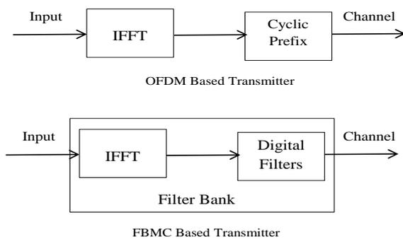
Figure 1: FBMC based Transmitter Design
