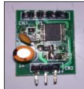
Figure 5. PWM dimming PCB
