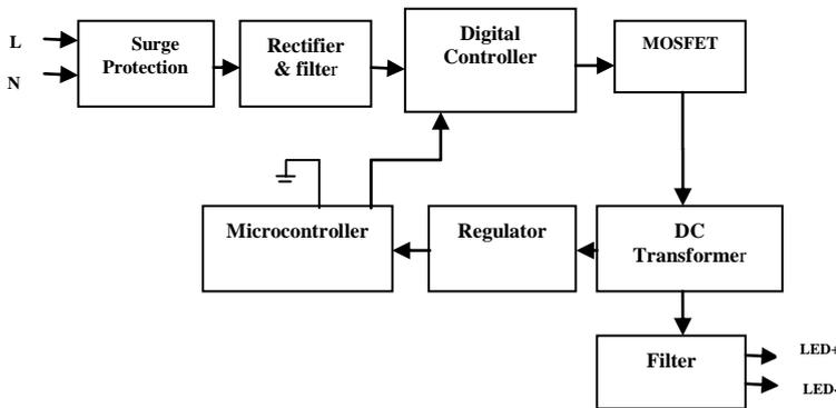
Figure 1. Block Diagram of Energy Efficient LED driver
