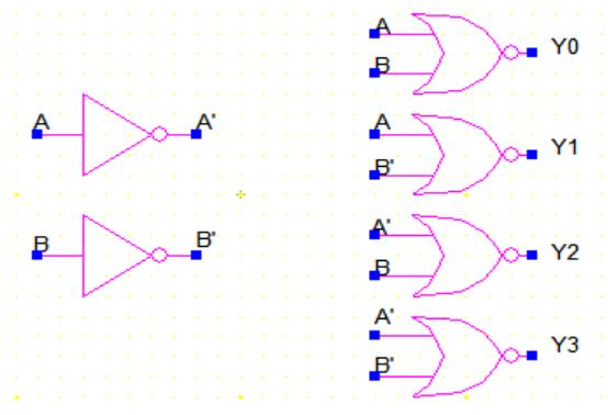
Figure 1. 20 transistor 2x4 decoder.
