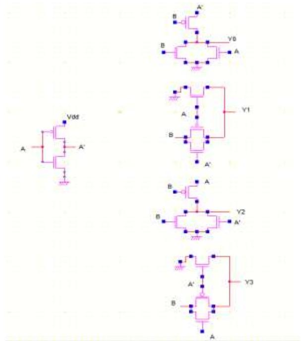
Figure 4. 14 transistor circuit for 2x4 Decoder
