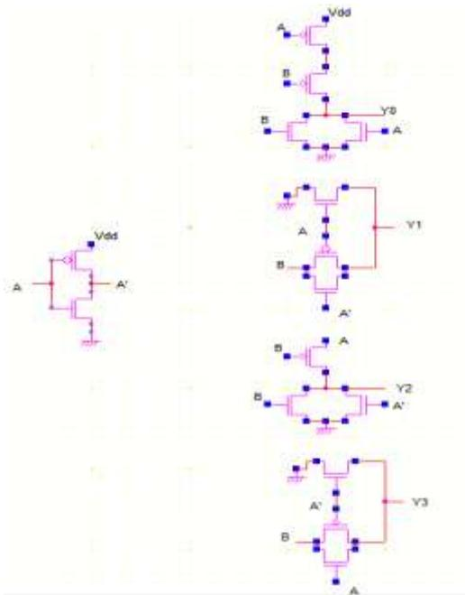
Figure 5. 15 transistor circuit for 2x4 Decoder
