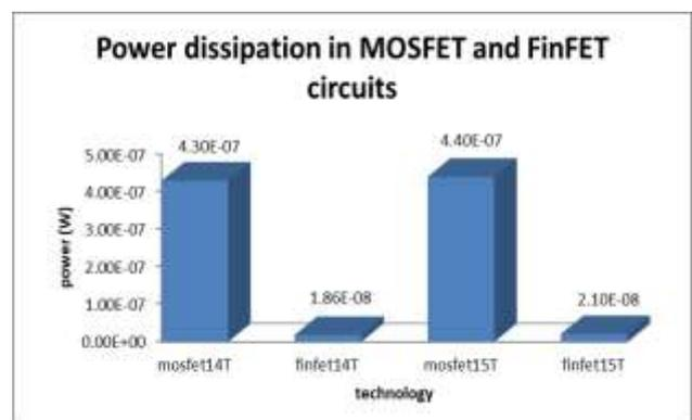
Figure 7: Power dissipation comparison
