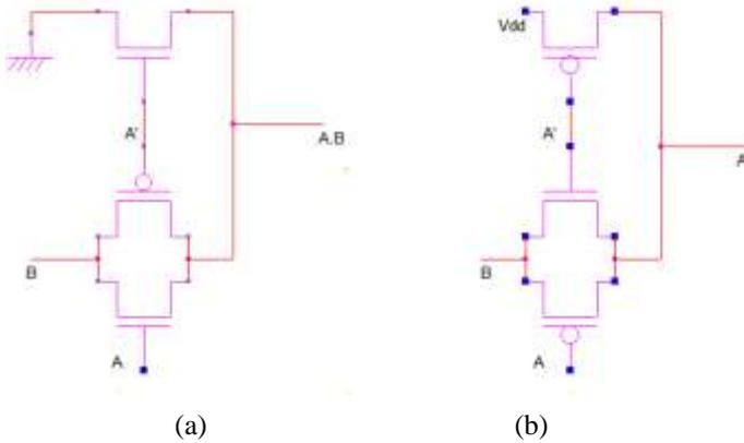
Figure 2. Three transistor TGL AND/OR gates used in decoder. (a) TGL AND gate (b) TGL OR gate
