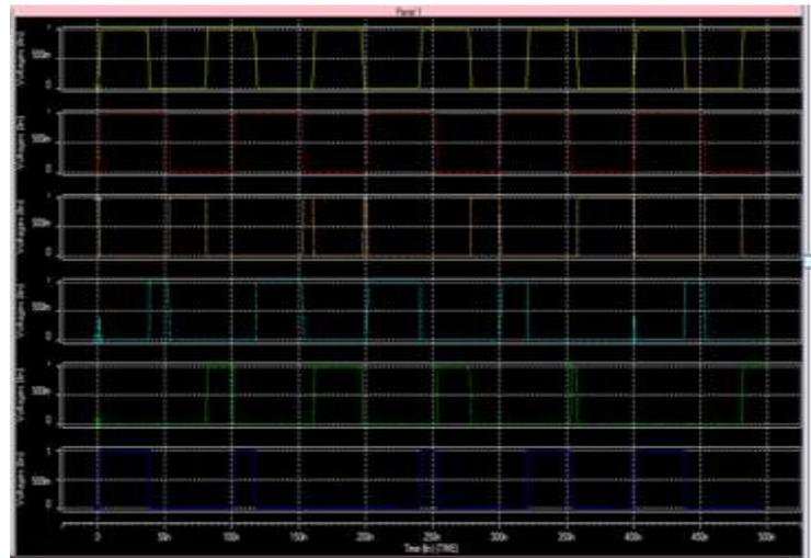
Figure 6: Output waveform for 2x4 decoder circuit.
