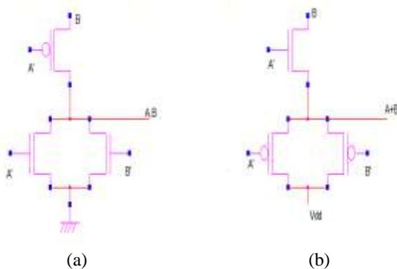
Figure 3. Three transistor DVL AND/OR gates used in decoder (a) DVL AND gate (b) DVL OR gate
