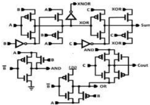
Fig. full-swing full adder cell
