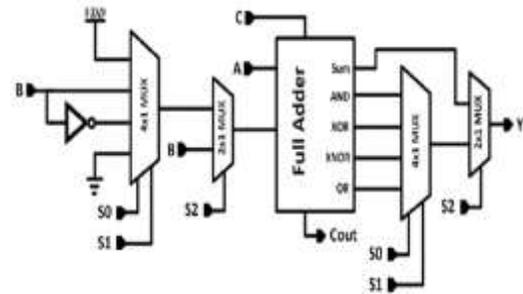
Fig.5.Schematic of 1 bit ALU Stage
