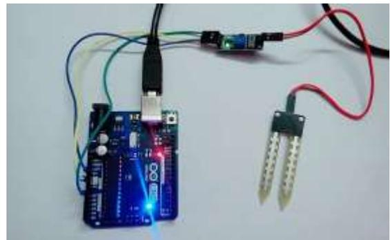
Figure8. Interfacing of Soil Moisture Sensor with Arduino
