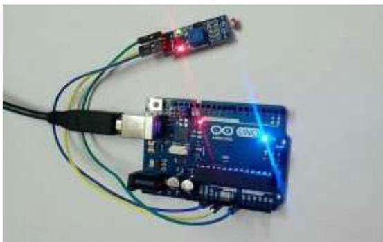
Figure6. Interfacing of Light Intensity Sensor with Arduino Sending light
