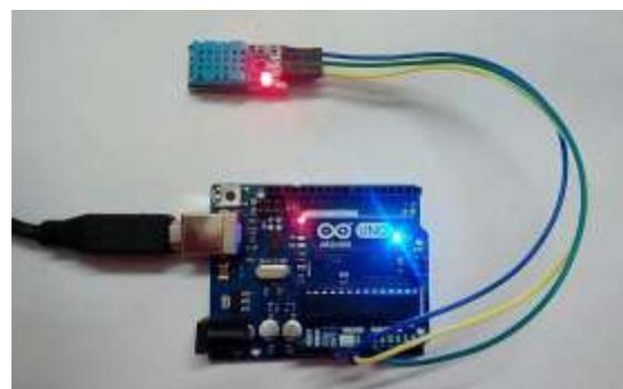
Figure4. Interfacing of DHT11 Sensor with Arduino Sending
