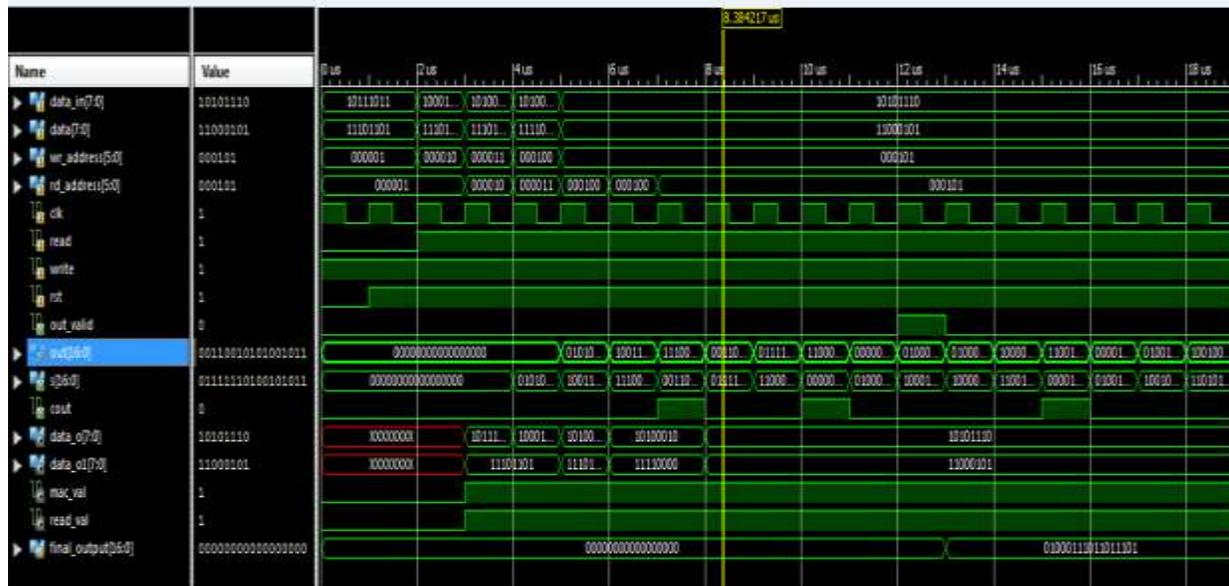
Fig 6 Simulation Result of CNN Accelerator
