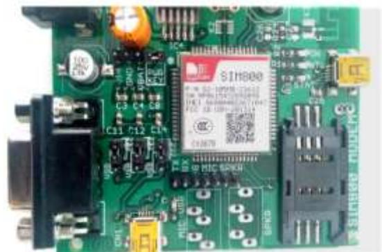
Figure 2.7: GSM modem
