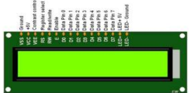
Figure 2.6: 16x2 LCD display
