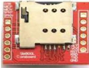
Figure 2.9: SIM card slot
