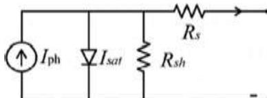
Figure 1. Equivalent circuit of the PV array
