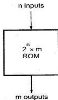
Figure 1: Block diagram of ROM
