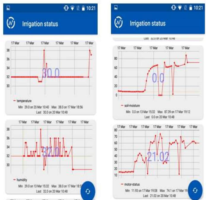
Figure 8: A view of the temperature, humidity value (Left), soil moisture and water level (Right) in the smart phone.
