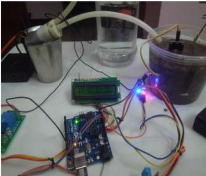
Figure 5: The relay stops the motor when the maximum is reached.
