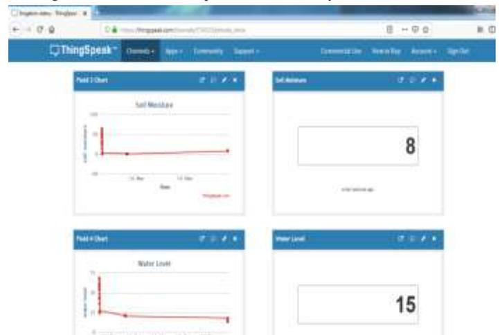
Figure 7: A view of the soil moisture and water level values in the website.
