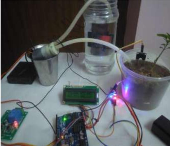
Figure 4: The relay signals the motor to start watering the plant when moisture level falls below the threshold.
