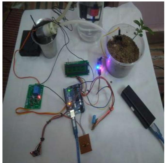
Figure 3: The hardware setup of the agricultural monitoring system
