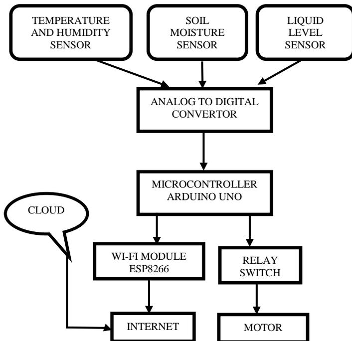
Figure 2: Block diagram of the agriculture monitoring system
