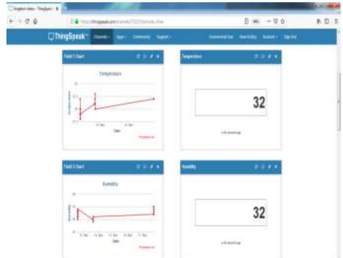
Figure 6: A view of the temperature and humidity values in the website.
