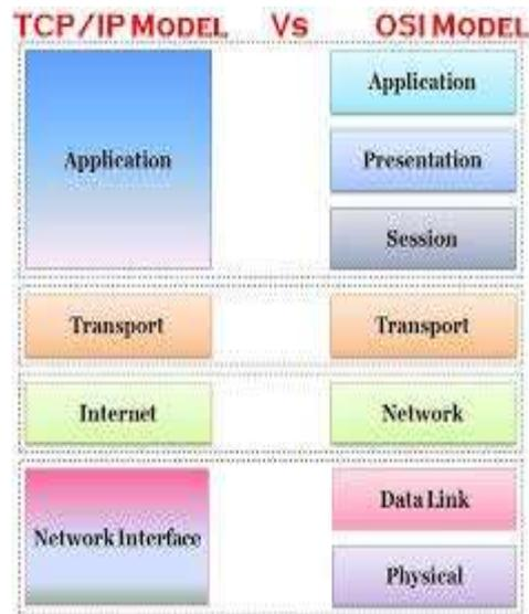
Figure4. Types of Network protocols VS OSI Model
