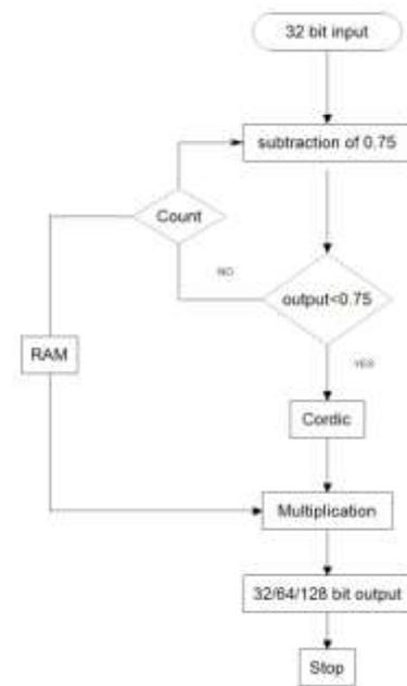
Figure5. Hardware flow to implement multiples other than 0.75.
