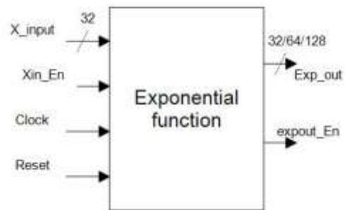
**Figure3.** The Pin Diagram of EFER
