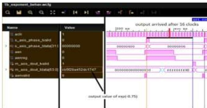
Figure6. Test Vector to show the Output for the value -0.75 Value
