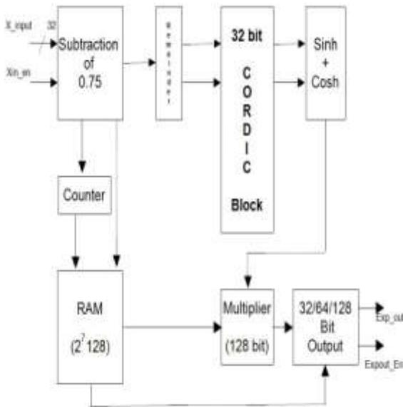
Figure4. VLSI Architecture of Extended Exponential Function.
