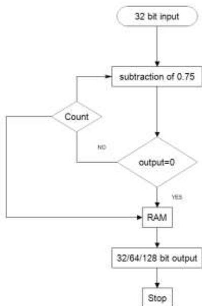
Figure5. Hardware flow to implement multiples of 0.75.
