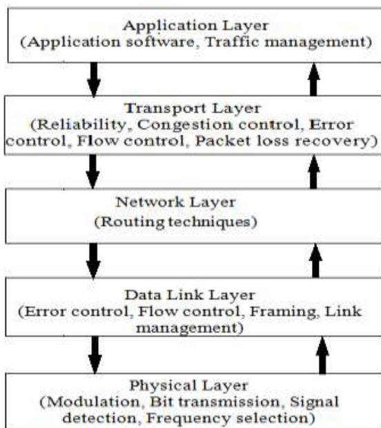
Fig 1 Wireless Sensor Networks Protocol Stack
