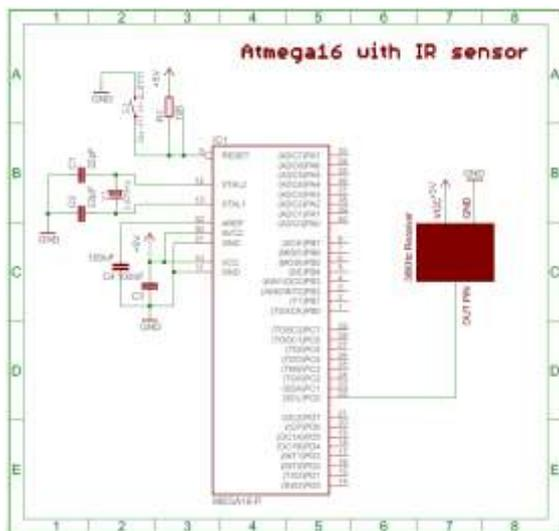
Fig -4: Modulated IR with Atmega16
