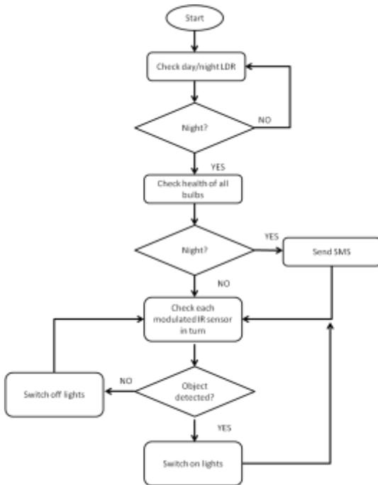
Fig -6: Flowchart for Atmega16 code
