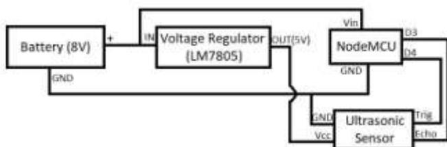
Figure 1 (a). Block diagram of the module.
