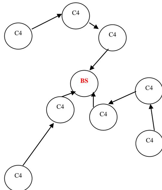
Fig. 5 Linear Routing Path for packet transfer by WSN.
