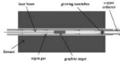
Figure 5 Laser ablation process
