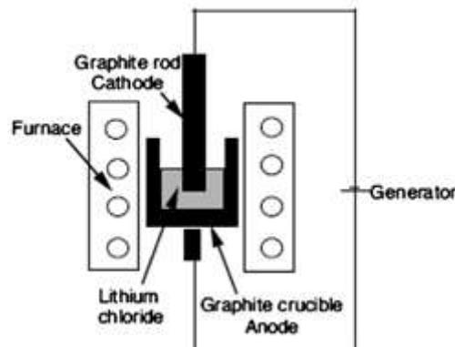
Figure 6 Electrolysis process
