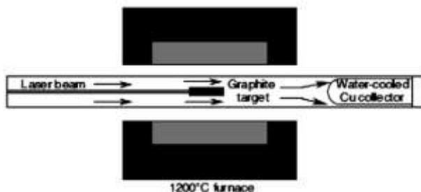
Figure 4 Laser-vaporization
