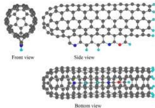
Figure 9. Three direction views of the closed end type carbon nanotube probe.
