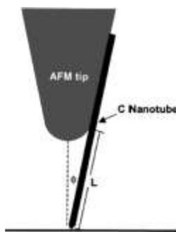
Figure 8 CNT attached to the tip of an AFM
