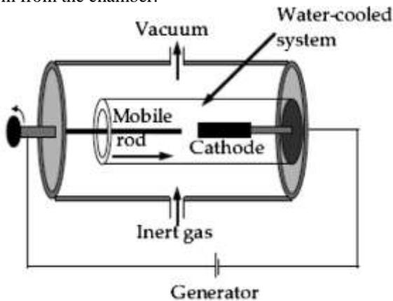
Figure3 Electric-arc method
