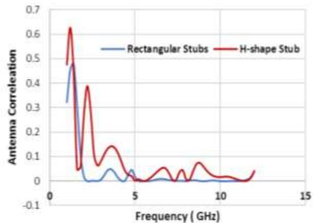
**Figure 3.** Simulated ECC plot for both stub designs
