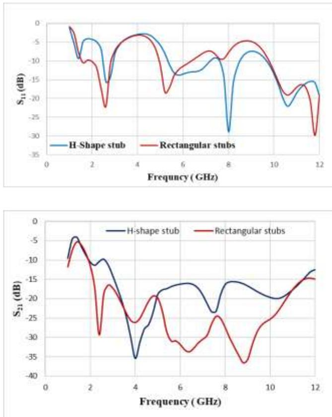
Figure 4. Simulated plots of (a)  $S_{11}$  plot for both proposed MIMO designs (b)  $S_{21}$  plot for both proposed MIMO designs
