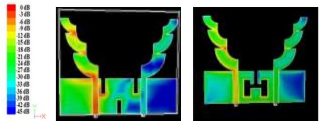
**Figure 2.** Surface Current Distribution a) Fractal MIMO antenna with three rectangular slots in ground plane b) Fractal MIMO antenna with H-shaped slot in ground plane
