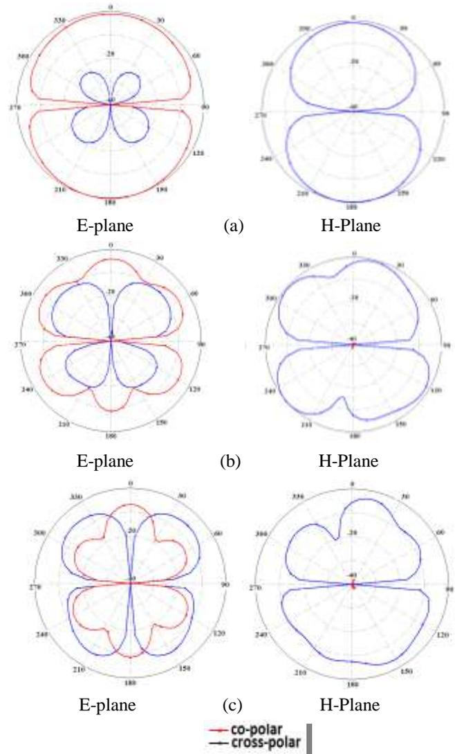
Figure 5. Simulated Radiation patterns for proposed antenna at (a) 2.6 GHz (b) 7 GHz and (c) 9.8GHz
