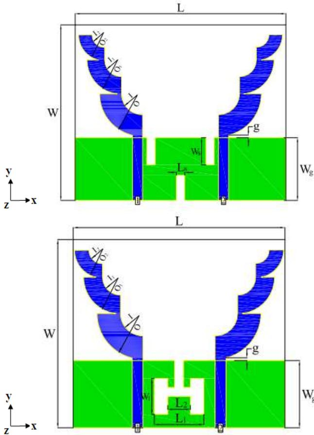
**Figure 1.** Antenna Geometries (a) Fractal MIMO antenna with three rectangular slots in ground plane (b) Fractal MIMO antenna with H-shaped slot in ground plane.
