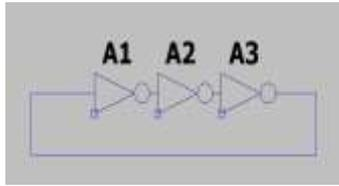
Figure 1 Voltage Controlled Ring Oscillator
