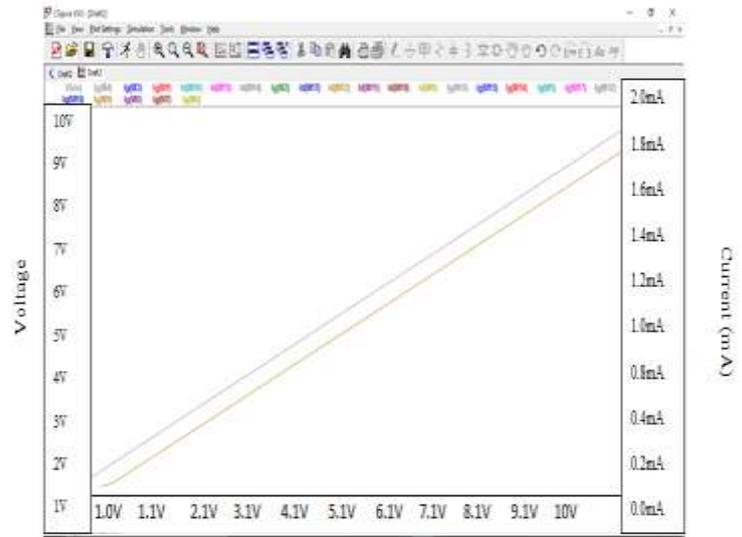
Figure 9 Voltage versus current response of VCO
