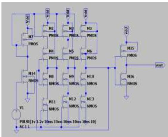
Figure 2 VCO design using a current starved method
