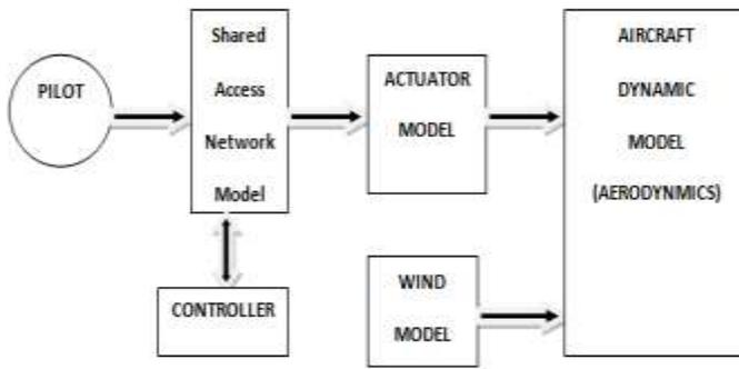
Figure1. Designing and analyzing the effect of communication delay or noise on flight control system.
