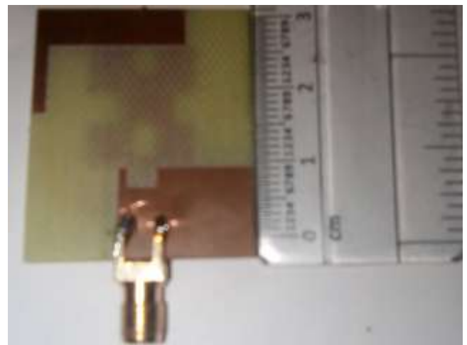
Figure 20. Fabricated ground view of the antenna
