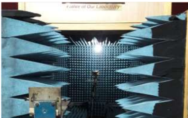
Figure 17. Isolated anechoic chamber to measure radiation pattern and gain
