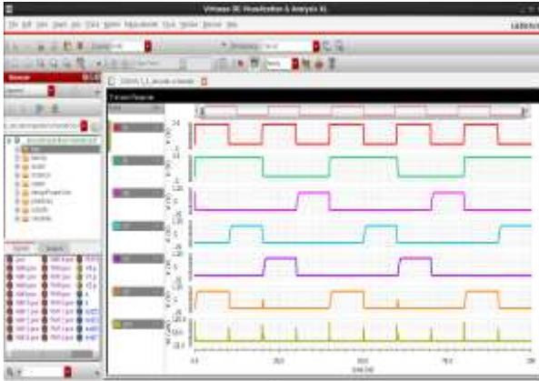
Figure 5: Proposed CMOS 2inputs and 4 outputs Decoder Output Waveform at 10MHz.
