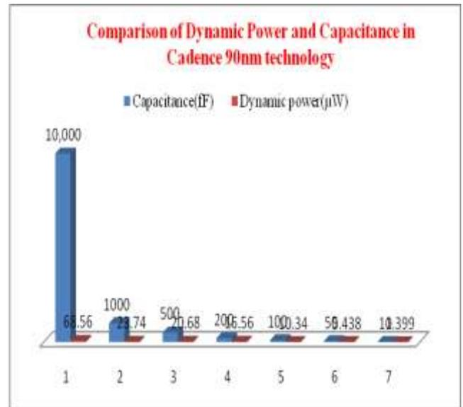
Figure 6: Comparison of Dynamic Power and Capacitance in Cadence 90nm technology
