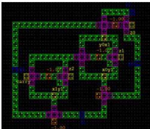
Figure 11.QCA Layout of Feynman Gate based 2x2 Array Multiplier
