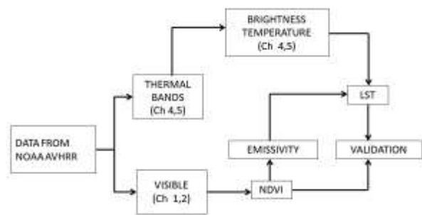
Figure2. Flow Diagram for retrieving LST from satellite data
