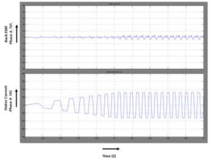
Figure 7a. Stator current and Back EMF of Phase 'A'
