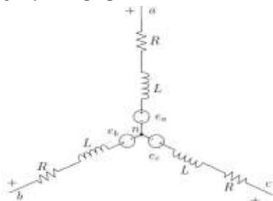
Figure 1. Electrical circuit of BLDC motor.
