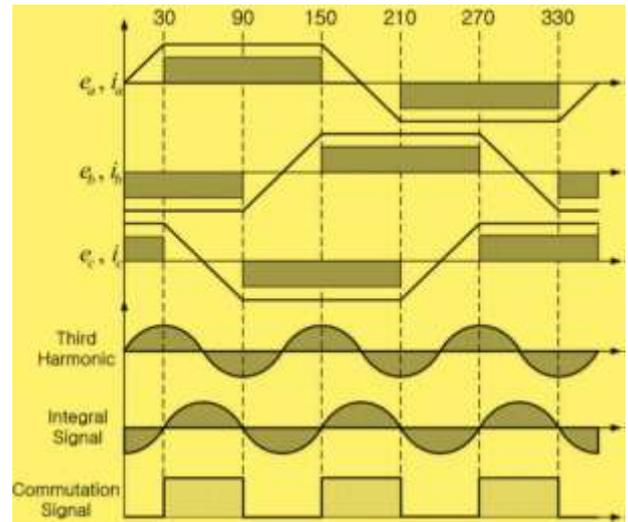
Figure 3. Trapezoidal waveforms with commutation signal using 3rd harmonic signals
