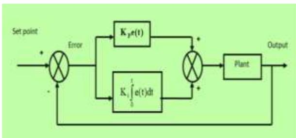
Figure 5. Structure of PI Controller
