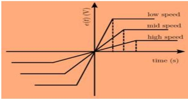
Figure 4. Integrated areas of the back-EMF signal
