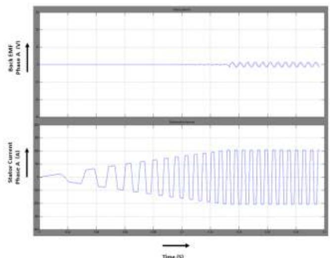
Figure 6a. Stator current and Back EMF of Phase 'A'
