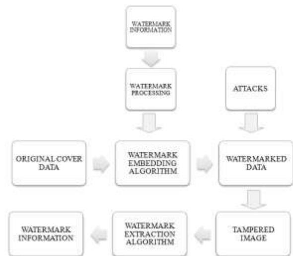
Figure1. Watermark embedding and extraction process in general.
