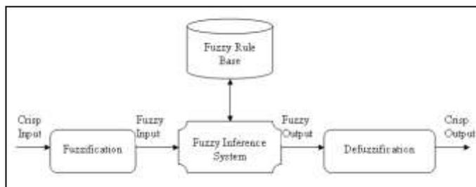
Figure 1. Fuzzy inference system architecture of UI
