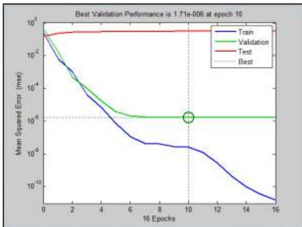
Figure 4(a). Mean square error of the model for Feed Forward Back Propagation with hidden neurons equal to 10
