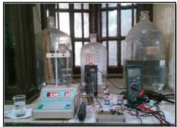
Figure 3. Experimental Setup for pH and conductivity measurement
