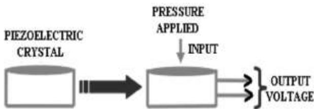
Figure2. Principle of piezoelectric effect
