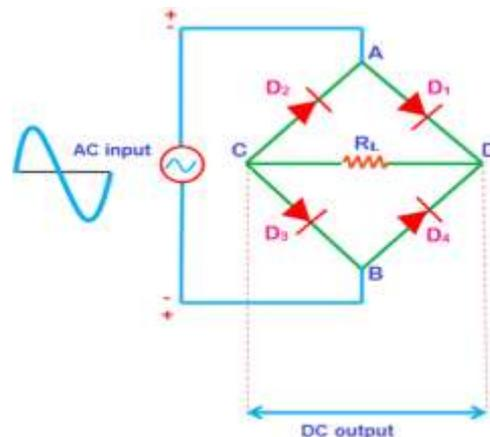
Figure3. Bridge Rectifier Principle
