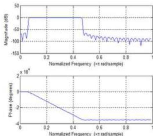
Figure 5: a) DC offset 4200 V removed using zero mean b) Magnitude and Phase response of filter
