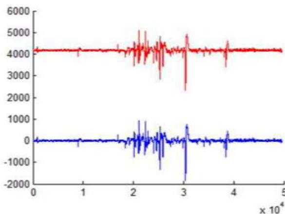
especially before performing any kind of analysis it is necessary to remove DC offset by subtracting the mean from the entire data of each electrode as shown in Figure 5.
