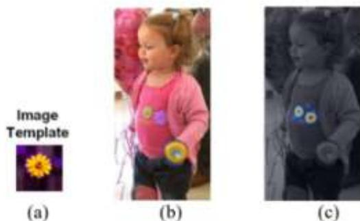
Figure1. (a)Template image (b) Reference image (c) Detected object superimposed on gray-scale image
