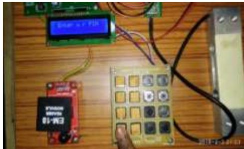
Figure 4. 4X4 Keypad Matrix to Enter Pin
