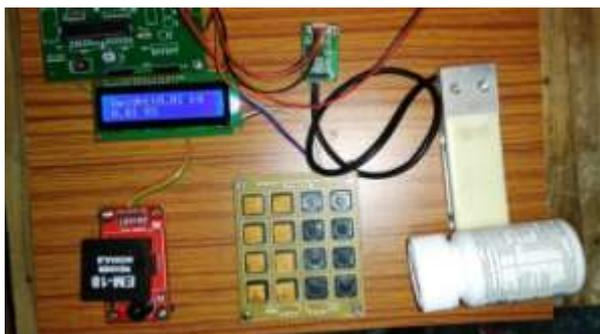
Figure 5 Weight Measurement Using Load Cell
