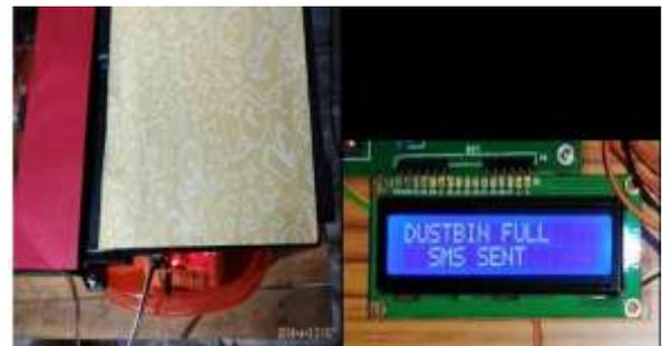
Figure 7. Detection of the Bin Level
