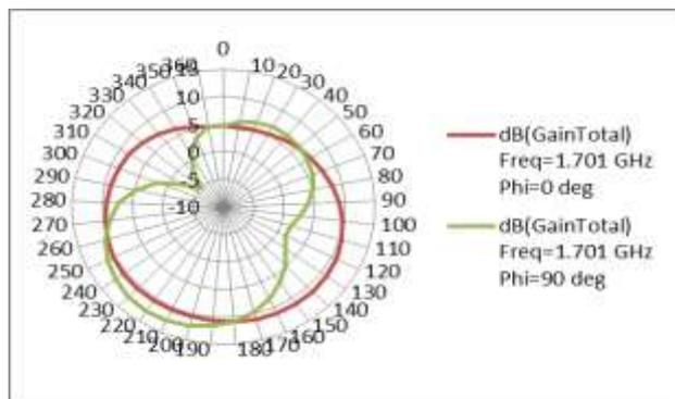
Figure 14. Radiation pattern of rectangular slot PIFA at frequency = 1.7010GHz
