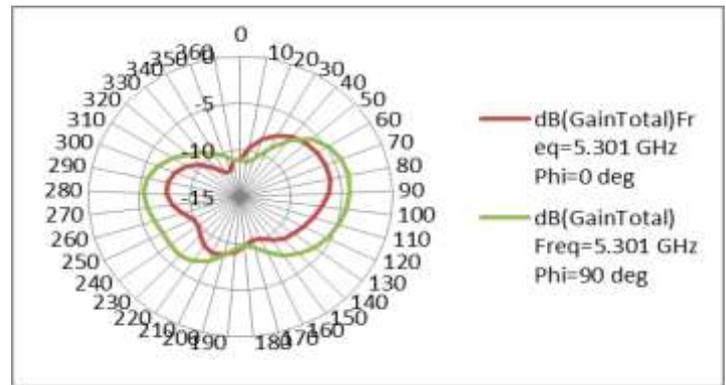
Figure 15. Radiation pattern of rectangular slot PIFA at frequency = 5.301GHz
