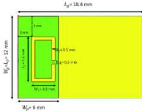
**Figure 2.** Top view of Proposed design 1
