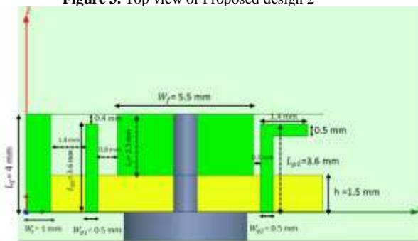
**Figure 4.** Side view of proposed design
