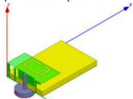
**Figure 5.** PIFA with a rectangular slot (3D view)
