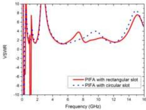
Figure 12. VSWR for rectangular and circular slot PIFA
