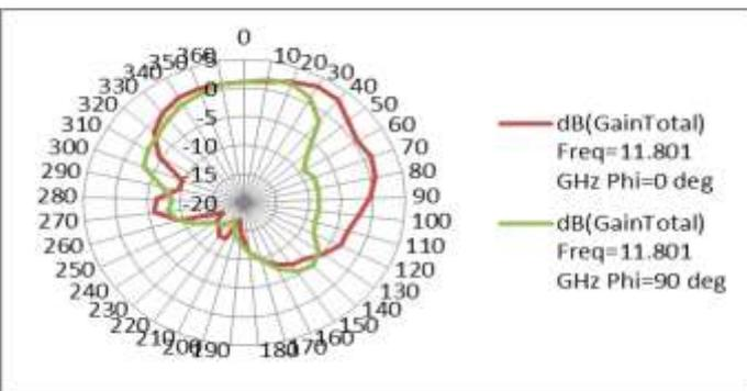
Figure 21. Radiation pattern of circular slot PIFA at frequency = 11.8010GHz
