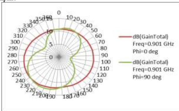
Figure 13. Radiation pattern of rectangular slot PIFA at frequency = 0.9010GHz
