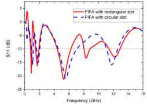
**Figure 9.** S11 parameter for rectangular as well as circular slot PIFA
