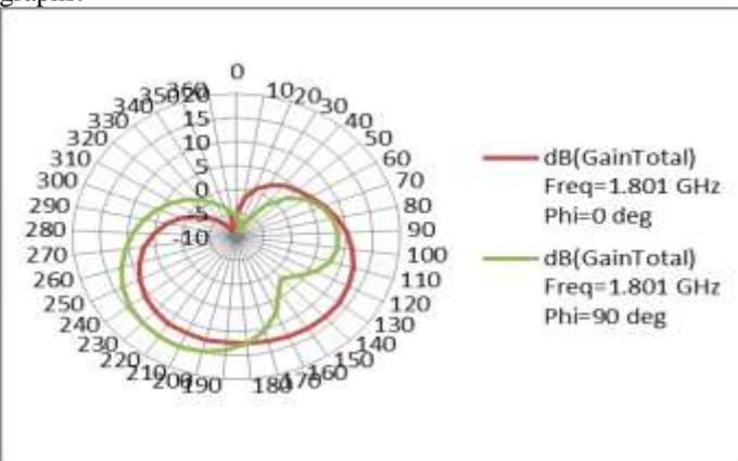
Figure 19. Radiation pattern of circular slot PIFA at frequency = 1.8010GHz
