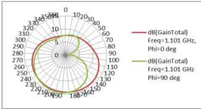
Figure 18. Radiation pattern of circular slot PIFA at frequency = 1.1010GHz
