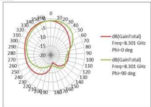
Figure 16. Radiation pattern of rectangular slot PIFA at frequency = 8.3010GHz
