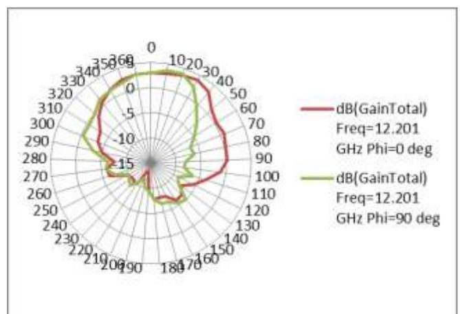
Figure 17. Radiation pattern of rectangular slot PIFA at frequency = 12.2010GHz
