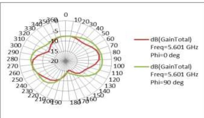
Figure 20. Radiation pattern of circular slot PIFA at frequency = 5.6010GHz
