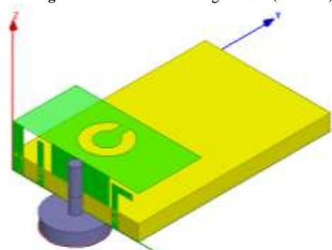
**Figure 6.** PIFA with a circular slot (3D view)
