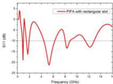
**Figure 7.** S11 parameter for rectangular slot PIFA
