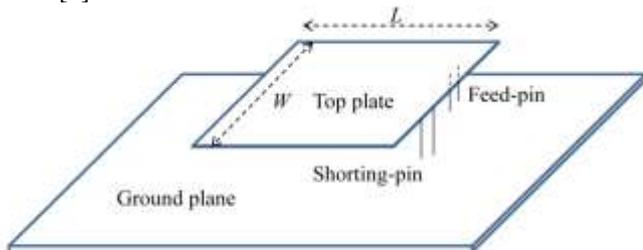
**Figure 1.** Basic structure of PIFA antenna [3]
