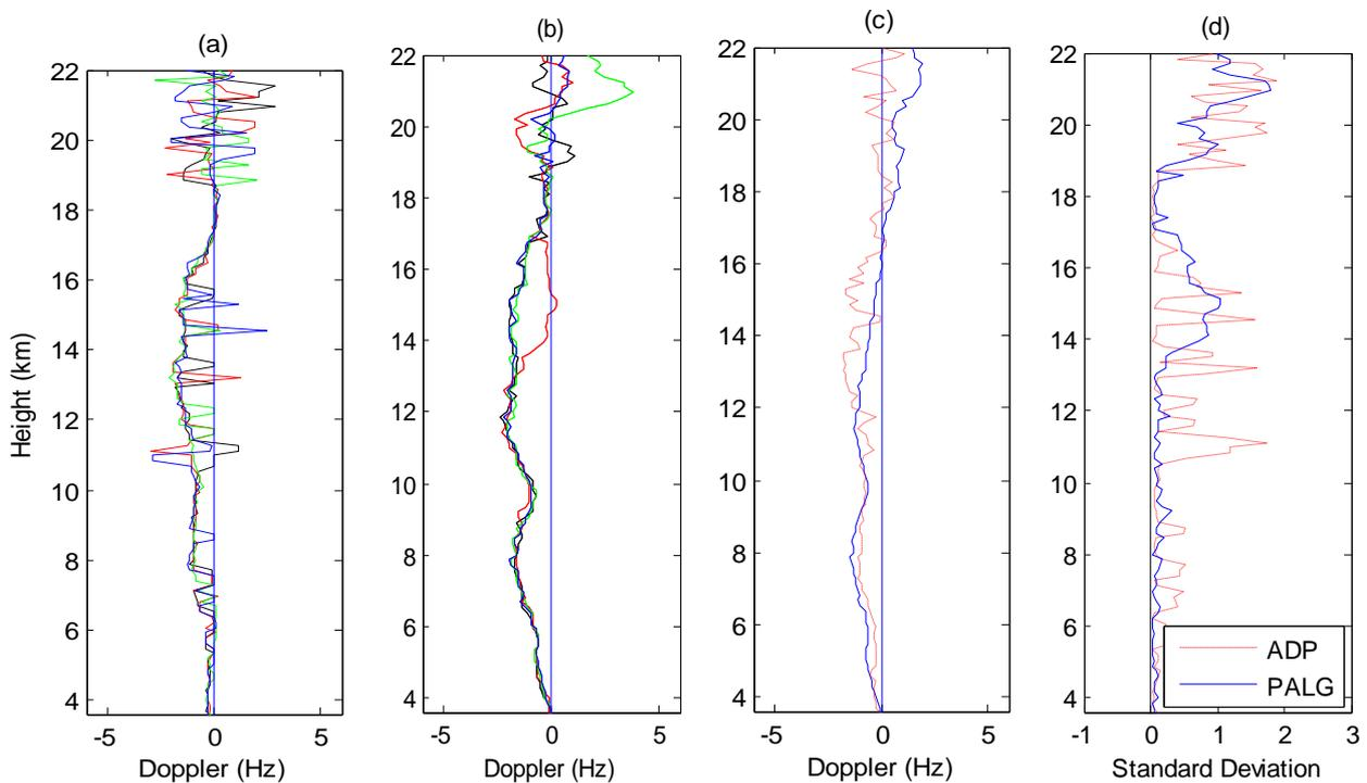
**Figure6.** Doppler height profiles for four scan cycles of the east beam using (a) ADP and (b) PALG. (c) Mean Doppler profile. (d) The standard deviation for the east beam of MST data Feb 10<sup>th</sup>, 2015.
