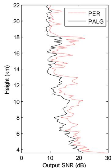
Figure 5. Height profiles of SNR estimated for the east beam of radar data.
