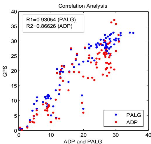
Figure 8. Correlation between ADP, PALG and GPS wind speeds for MST data.
