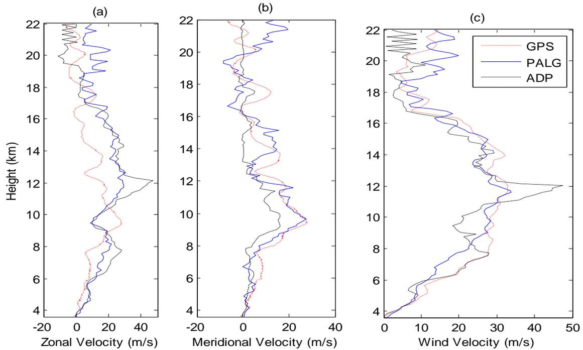
Figure 7. Wind speed comparisons for the radar data collected on Feb 10<sup>th</sup>, 2015 using ADP, PALG and GPS.
