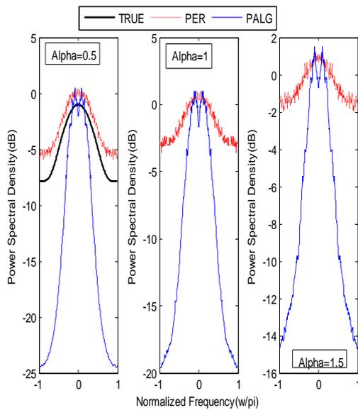
Figure 2. Estimation of Power spectral density (PSDs) using PALG and PER in presence of noise associated with amplitudes  $\alpha=0.5$ ,  $\alpha=1$  and  $\alpha=1.5$ .
