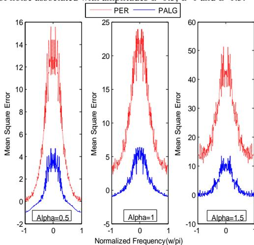
Figure 3. Estimation of Mean Square Error (MSEs) using PALG and PER in presence of noise associated with amplitudes  $\alpha=0.5$ ,  $\alpha=1$  and  $\alpha=1.5$ .
