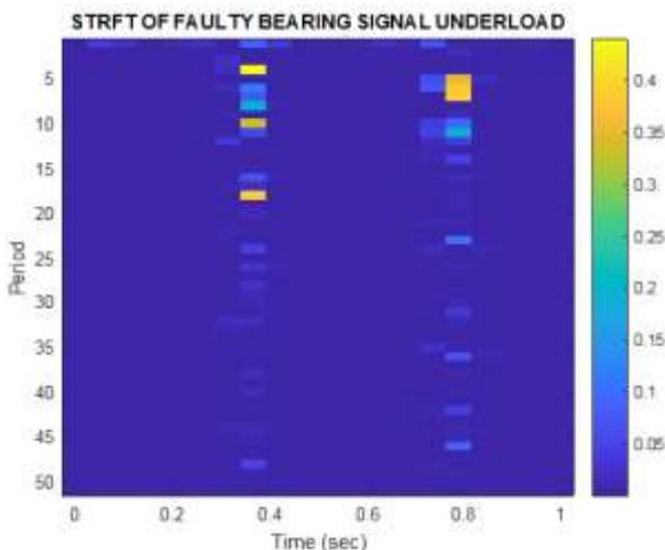
Figure14. ST-RFT of faulty time signal
