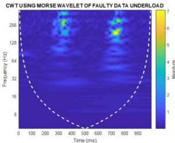
Figure13. Scalogram of faulty time signal
